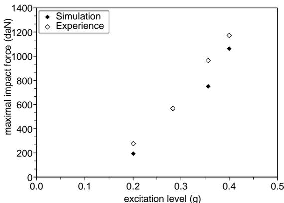
Figure 7: Comparison of the maximal impact force for different excitation level, in water
