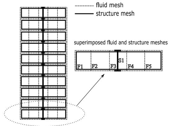
Figure 4: Fluid and structure mesh used to discretize one fuel assembly
