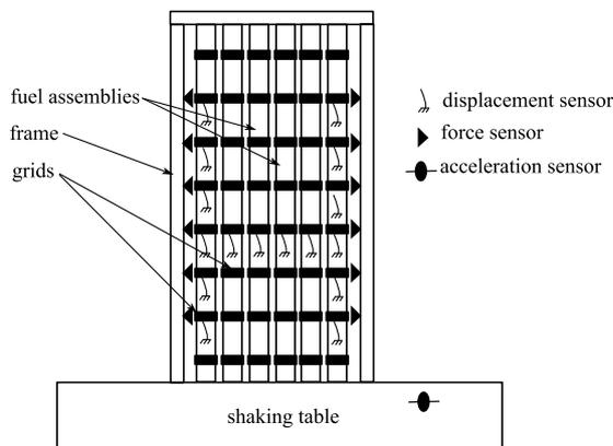
Figure 5: Experimental device
