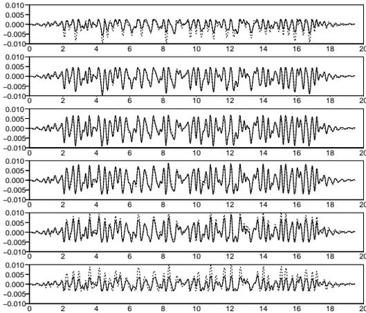
Figure 6: Relative displacements of the fourth grids of the fuel assemblies (m) vs time (s), comparison simulation (continuous line) experimental data (dash line), in water with 0.4 g excitation level
