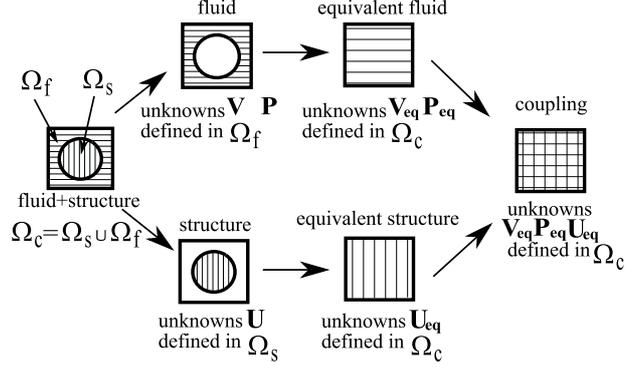
Figure 1: Porous modelling and method
