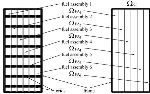
Figure 2: Modelling of six fuel assemblies
