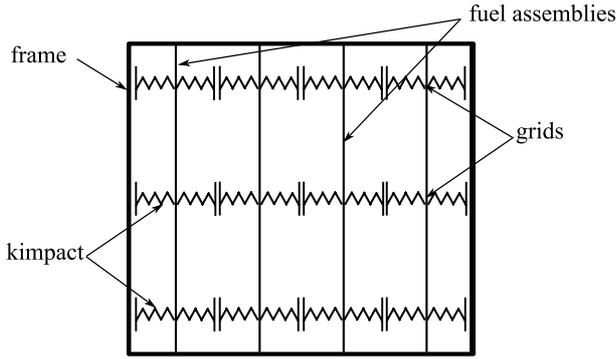
Figure 3: Impact model for four fuel assemblies with three grids
