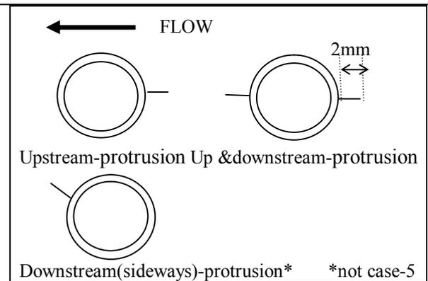
Fig.3 Measured cylinder arrays with projection
