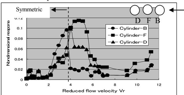
Fig.7 Three cylinders in tandem (Normal surface)
