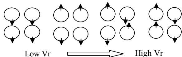
Fig.14 Vibration mode of cylinders
