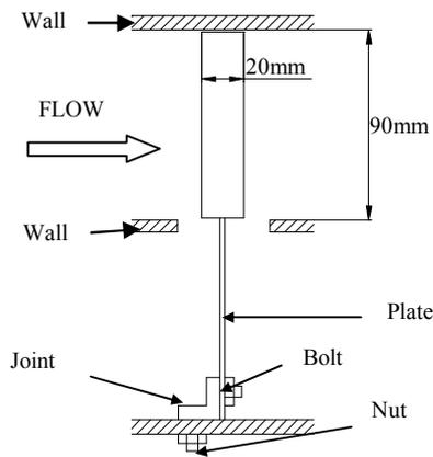
Fig.2 Concept of test cylinders
