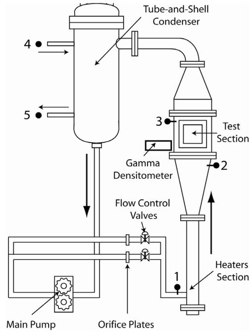
Figure 2: Two-Phase Flow Loop
