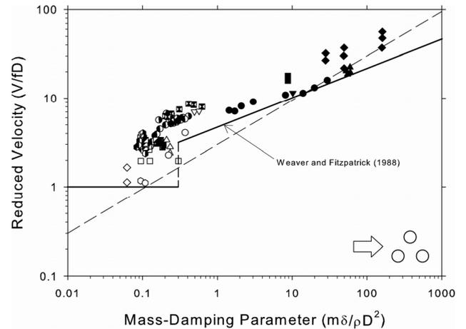
Figure 5: Stability map based on damping in quiescent fluid. The reduced velocity is based on the pitch velocity for single-phase data and the interfacial velocity for two-phase data.
