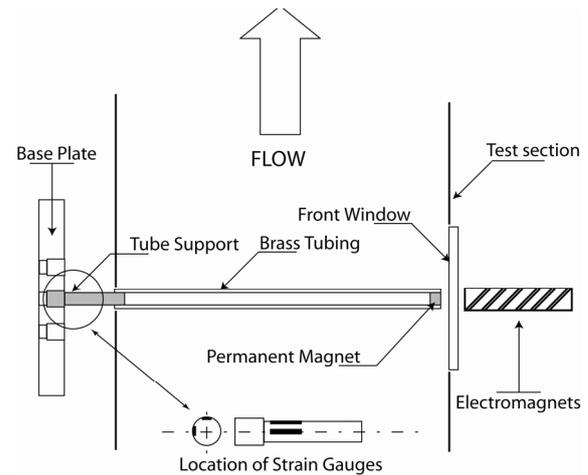
Figure 3: Schematic diagram of the model tube showing the strain gauges and the electromagnets.
