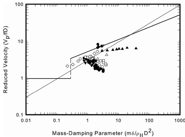
Figure 1: *Stability Map for fluidelastic instability in two-phase flows*
