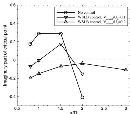
Figure 2: Stability analysis: Imaginary part of the critical point as a function of the streamwise location in the cylinder wake (positive values denoting absolute instability, negative values denoting convective instability).
