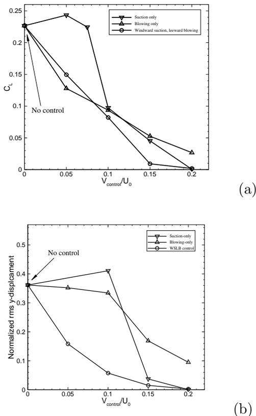
Figure 1: Lift/VIV reduction: (a) *r.m.s.* lift coefficient  $C_L$  as a function of the normalized control velocity  $V_{control}/U_0$  for the stationary case. (b) *r.m.s.* cylinder displacement in cross-flow direction as a function of control velocity for a freely vibrating cylinder subject to VIV.
