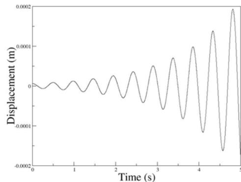
Figure 6 : Example of tube displacement time history for an inlet velocity of  $0.3 \text{ m.s}^{-1}$  with structure parameters of Table 3.
