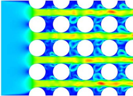
Figure 9 : Example of flow field for an inlet velocity of  $0.075 \text{ m.s}^{-1}$  with structure parameters of Table 4 (Huvelin 2008).
