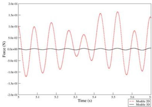
Figure 11 : Comparison of fluid forces acting on the moving tube estimated by two-dimensional and three-dimensional computations (Huvelin 2008).
