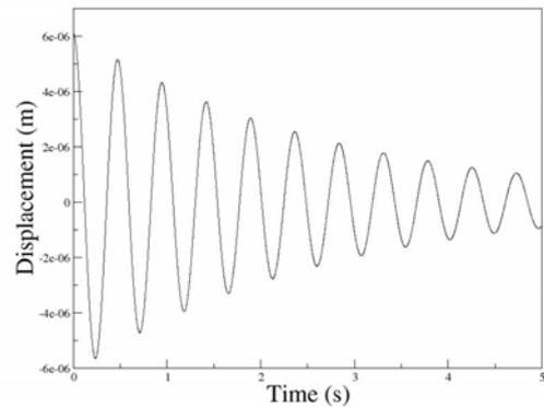
Figure 5 : Example of tube displacement time history for an inlet velocity of  $0.015 \text{ m.s}^{-1}$  with structure parameters of Table 3.
