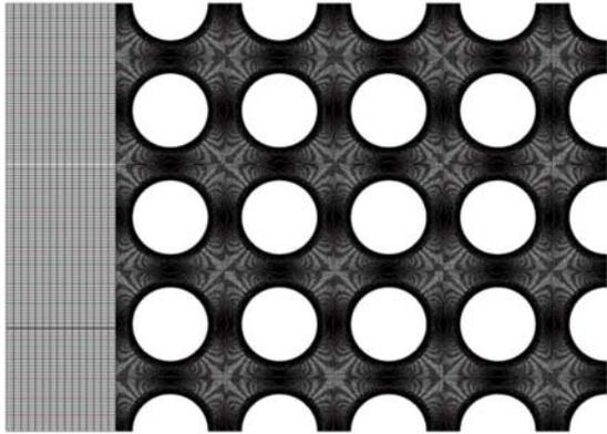
Figure 3 : Example of fluid domain mesh.
