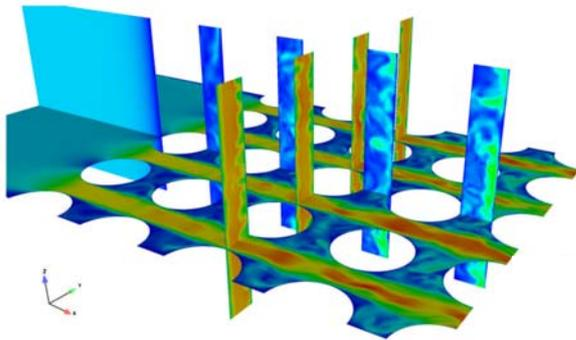
Figure 10 : Flow three-dimensional effects for an inlet velocity of  $0.075 \text{ m.s}^{-1}$  with structure parameters of Table 4 (Huvelin 2008)
