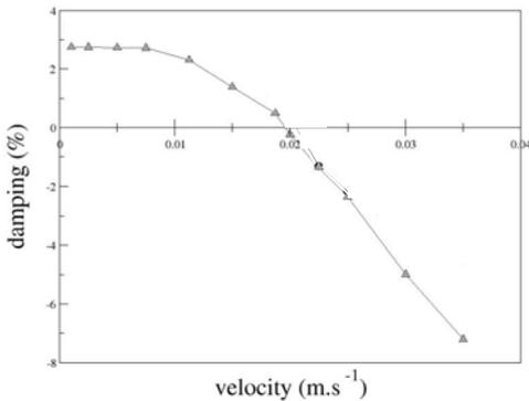
Figure 8 : Tube vibration damping in terms of flow inlet velocity with structure parameters of Table 3 (Huvelin 2008).
