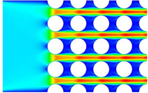
Figure 4 : Example of fluid flow field for an inlet velocity of  $0.015 \text{ m.s}^{-1}$  with structure parameters of Table 3.
