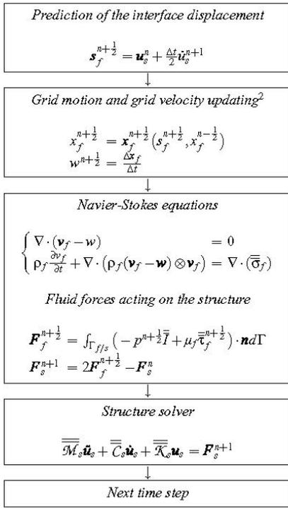
Figure 1 : Computational procedure for simulation of a fluid structure coupled problem.
