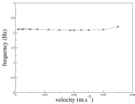
Figure 7 : Tube vibration frequency in terms of flow inlet velocity with structure parameters of Table 3 (Huvelin 2008).
