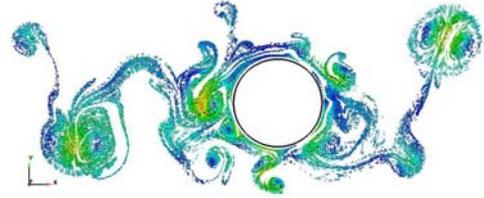
Figure 2: Instantaneous flow pattern around oscillating cylinder.
