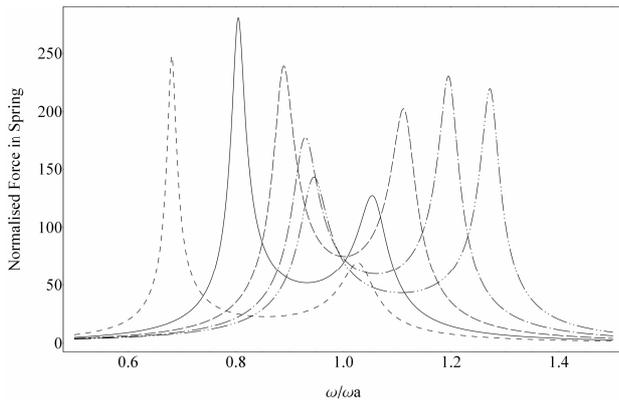
Figure 2. Frequency response functions for coupled system with  $\zeta_s = 0.01$ ,  $\zeta_a = 0.03$ ,  $\beta = 0.013$  and  $\omega_s/\omega_a = \text{---} 0.7$ ,  $\text{---} 0.849$ ,  $\text{- - -} 0.988$ ,  $\text{- \cdot - \cdot} 1.11$ ,
