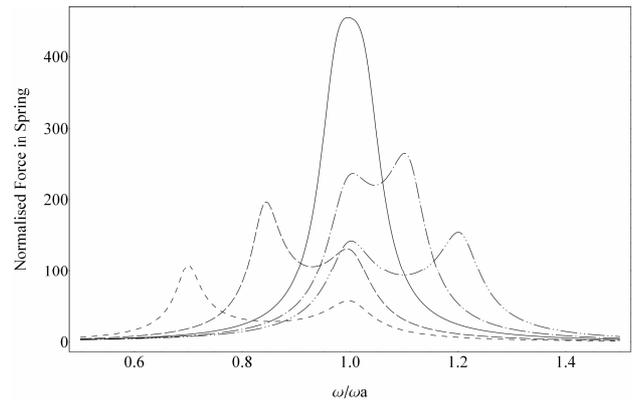
Figure 3. Frequency response functions for coupled system with  $\zeta_s = 0.03$ ,  $\zeta_a = 0.04$ ,  $\beta = 0.001$  and  $\omega_s/\omega_a = \text{---} 0.7$ ,  $\text{- - -} 0.845$ ,  $\text{---} 1.0$ ,  $\text{- \cdot - \cdot} 1.1$ ,
