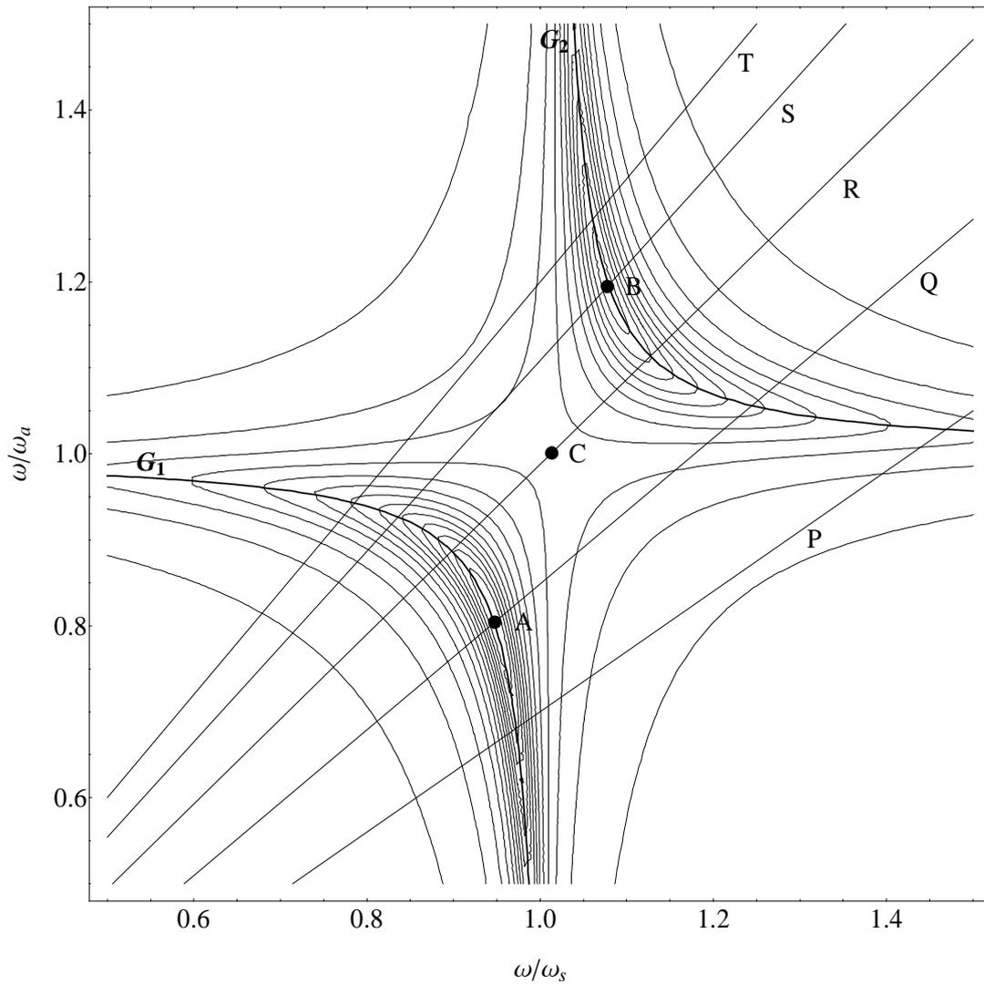
Figure 4. Contours of Equation 9 on a two-dimensional frequency plot. Sections along the lines P, Q, R, S and T correspond to the curves in Figure 2. The global maxima is at A with a second peak at B and a saddle at C. Lines  $G_1$  and  $G_2$  correspond to the locus of natural frequencies of the undamped coupled system.
