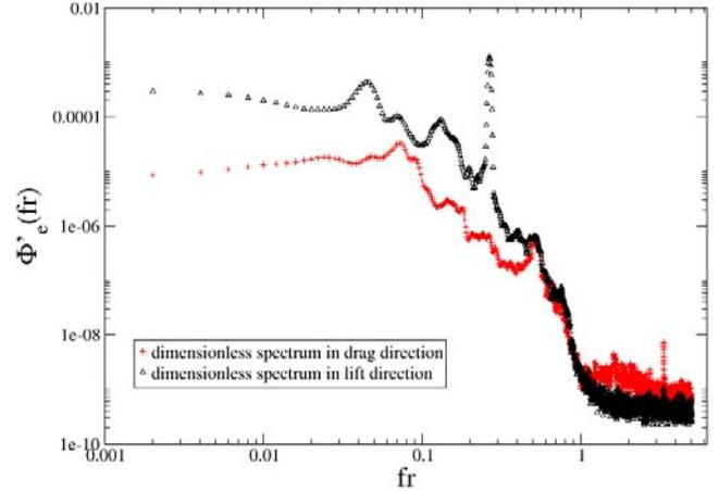
Figure 5 : Dimensionless spectra (in drag and lift directions) versus reduced frequency with  $Re=121500$
