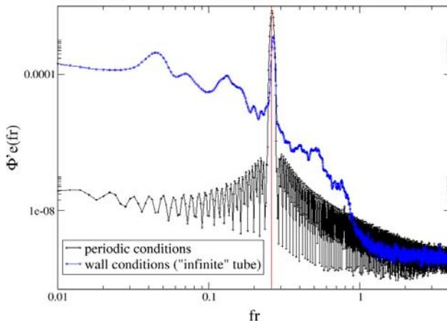
Figure 7 : Influence of boundary conditions on dimensionless spectrum in lift direction
