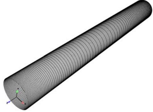
Figure 2 : Tube wall surface mesh
