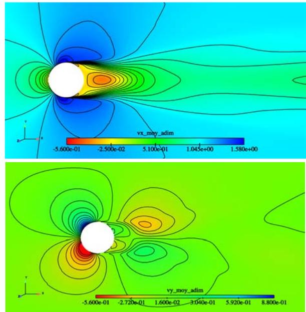
Figure 4 : Computation results : components of mean velocity along drag (upper graph) and lift directions (lower graph)
