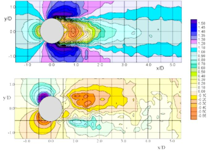
Figure 3 : Braza’s Particle Image Velocimetry measurements : components of mean velocity along drag (upper graph) and lift directions (lower graph)
