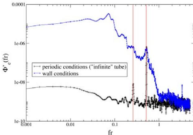
Figure 6: Influence of boundary conditions on dimensionless spectrum in drag direction
