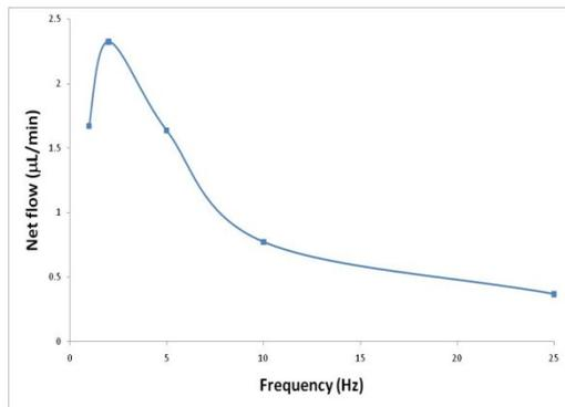
**Figure 6:** Plot of the net flow pumped through the micropump for different actuating frequencies
