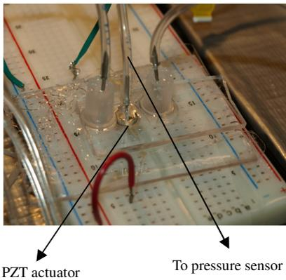
**Figure 3:** Chamber pressure measurement setup for micropump
