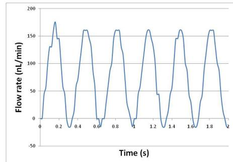
**Figure 5:** Flow rate vs. Time for a pumping frequency of 3 Hz
