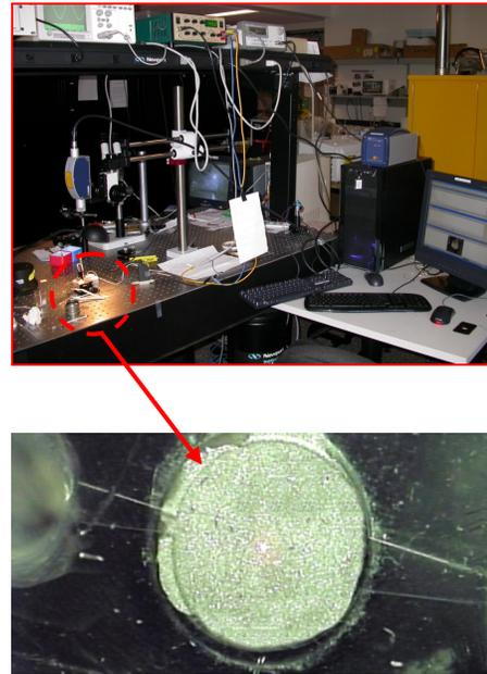
**Figure 1:** Experimental setup for the measurement of pump deflection using a single point Laser Doppler Vibrometer
