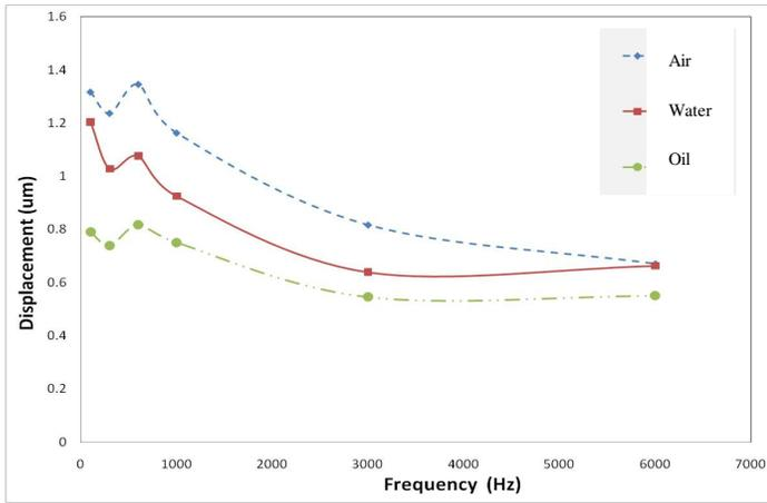
**Figure 2:** Plot of central pump deflection at different operating frequencies in different media
