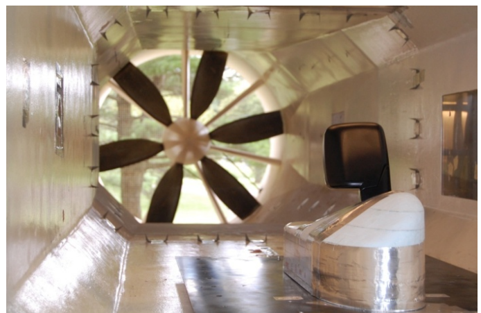
Figure 3 Mounting of the side view mirror looking downstream
