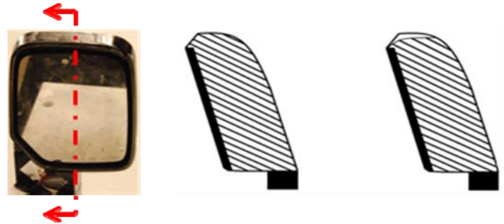
Figure 2 Cross sections of the mirrors Baseline (left) - Turn Signal (right)
