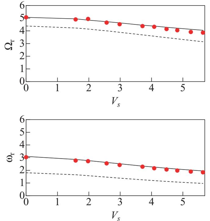
**FIGURE 4.** The natural frequency  $\Omega_r$  and  $\omega_r$  as functions of flow velocity for the first mode ( $\alpha = 0.667$ ,  $\beta = 0.401$ , solid line: theoretical result  $\gamma = 4.22$ , broken line: theoretical result  $\gamma=0$ ,  $\bullet$ : experimental result)
