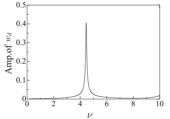
**FIGURE 7.** Frequency response curve of amp. of  $w_d$  ( $V_s=3.68, \varepsilon=0.05, c_w=0.091$ )
