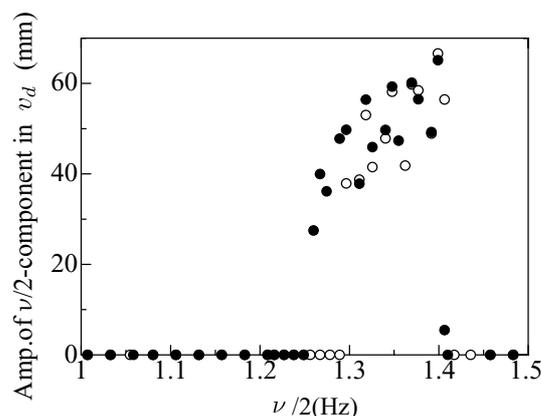
FIGURE 16. Frequency response of the out-of-plane vibration (○:forward sweep of  $\nu$ ,●:downward sweep of  $\nu$ )
