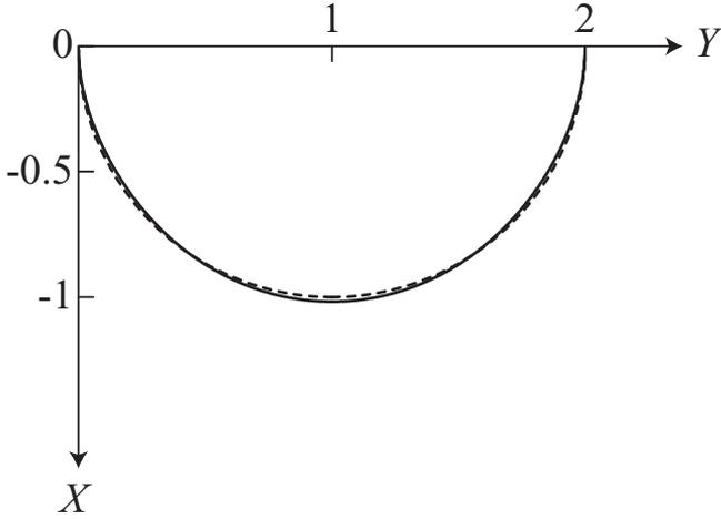
**FIGURE 3.** Static equilibrium state of the curved pipe ( $V_s=3.68, \gamma=4.22$ , solid line: static equilibrium state, broken line: semicircle)
