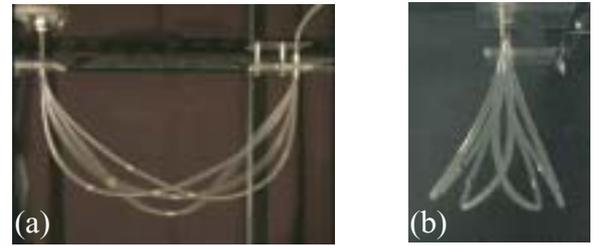
FIGURE 13. Photographs of the spatial behavior of the curved pipe, (a): in-plane vibration, (b): out-of-plane vibration
