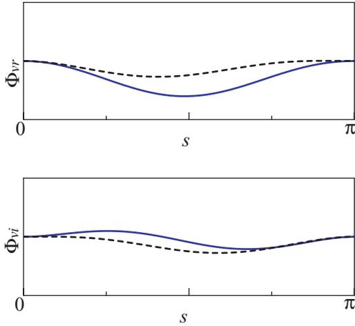
**FIGURE 5.** First mode shape  $\Phi_v$  ( $V_s=3.68$ , solid line:  $\gamma=4.22$ , broken line:  $\gamma=0$ )
