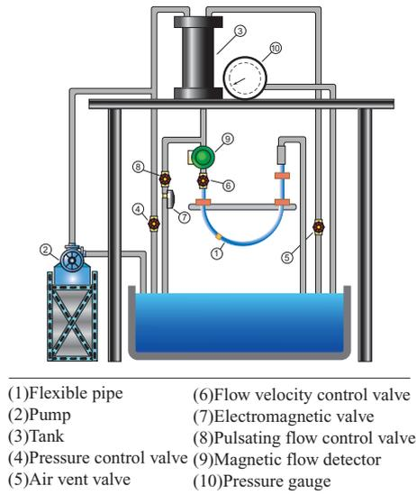
FIGURE 11. Diagram of experimental setup
