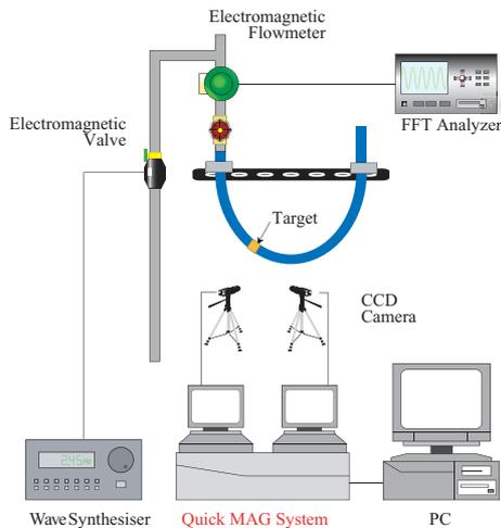
FIGURE 12. Measurement system of spatial pipe displacements
