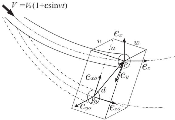
FIGURE 2. Deformation of a Curved Pipe
