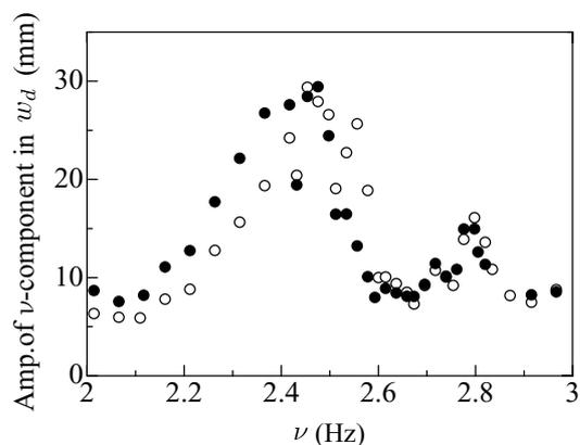
FIGURE 15. Frequency response of the in-plane vibration (○:forward sweep of  $\nu$ ,●:downward sweep of  $\nu$ )
