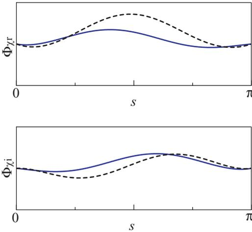
**FIGURE 6.** First mode shape  $\Phi_\chi$  ( $V_s=3.68$ , solid line:  $\gamma=4.22$ , broken line:  $\gamma=0$ )
