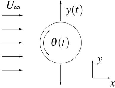
**FIGURE 1.** Schematic showing the problem geometry and important parameters relevant to the combined forced oscillation and the circular cylinder model. The streamwise direction is the  $x$ -direction.
