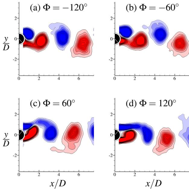
**FIGURE 3.** Motion phased-locked vorticity contours taken at the motion-phase of  $t = T$  for  $f_N=0.6$  Hz,  $F_R=1$ ,  $A_t = D/4$ ,  $A_\theta = 0.5$  radian and  $Re_{avg} = 1322$ . The near-wake vorticity is shown for different  $\Phi$  values. The flow direction is from left to right. Vorticity contours are evenly spaced over the range  $[-0.1 : 0.1]$ ; with  $\Delta\omega_{zrms} = 0.01$ .
