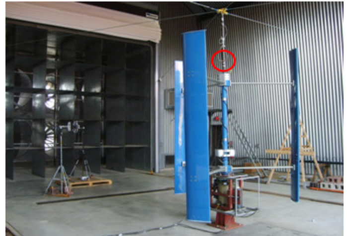
Figure 4: Wind turbine mounted within the wind tunnel. Highlighted region indicates the accelerometer mounting location. Note the sonic and propeller type anemometers located upstream of the turbine as well as the guy wire support system attached to the top of the turbine's stationary inner shaft.
