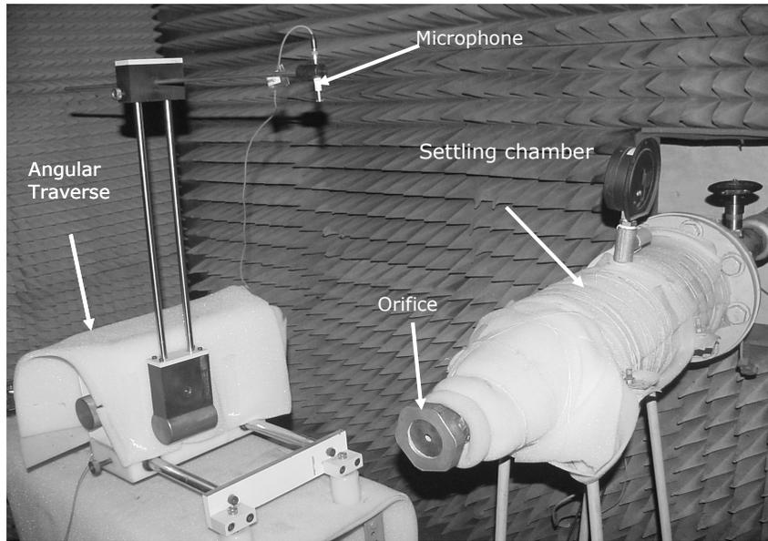
FIG.3 PHOTOGRAPH SHOWING THE ARRANGEMENT OF TRAVERSE MECHANISM
