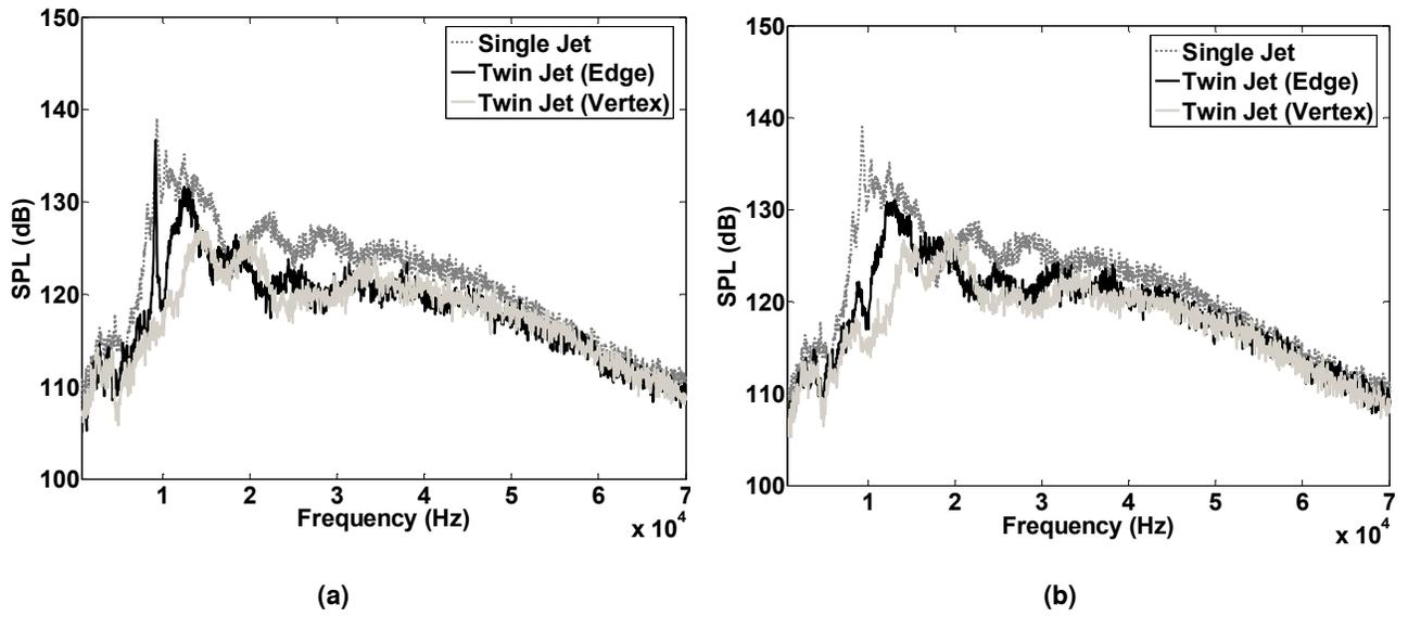
FIG.5 SPECTRA FROM SINGLE AND TWIN JETS FOR NPR = 7, S/D = 0.5 (a)  $\theta = 90^\circ$ ; (b)  $\theta = 0^\circ$ .
