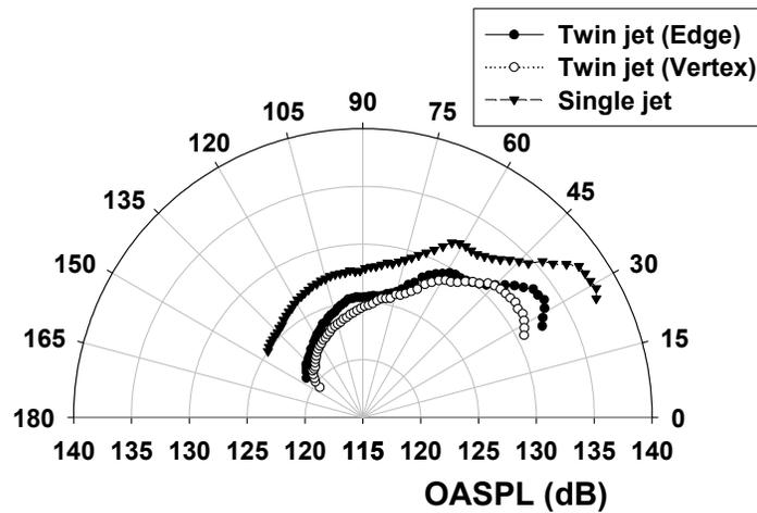
FIG. 8 OASPL OF SINGLE AND TWIN JETS FOR NPR = 7,  $S/D = 0.5$
