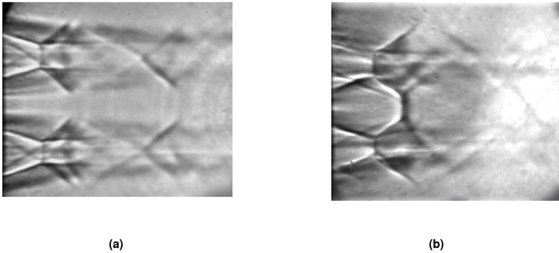
FIG. 6 SHADOWGRAPH IMAGES OF PLUME COUPLING: a) NO COUPLING; b) COUPLING
