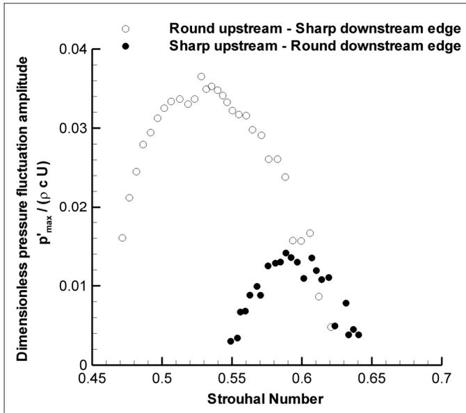
Figure 8: Measured dimensionless pressure fluctuation amplitude for the 3<sup>rd</sup> acoustic mode as a function of Strouhal number for *round upstream - sharp downstream* ( $r_{up}/W = 0.1$ ) case and *sharp upstream - round downstream* ( $r_{down}/W = 0.1$ ) case. (Nakiboglu *et al.* [15])
