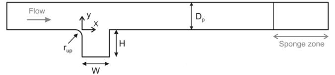
**Figure 3: Computational domain and relevant parameters.**
