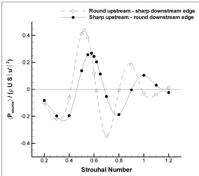
Figure 9: Calculated dimensionless average acoustic source power  $\langle P_{source} \rangle / \rho U S |u'|^2$  as a function of Strouhal number for *round upstream - sharp downstream* ( $r_{up}/W = 0.25$ ) edge and *sharp upstream - round downstream* ( $r_{down}/W = 0.25$ ) edge configurations with a perturbation amplitude of  $|u'_{\max}|/U = 0.05$ .
