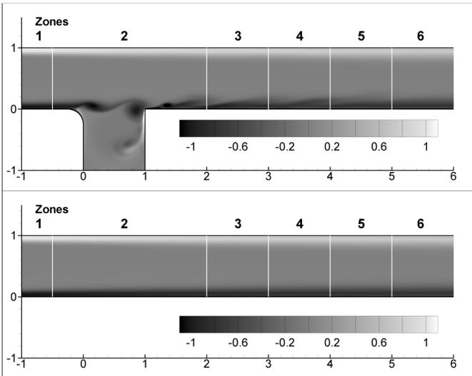
**Figure 5: Normalized vorticity contours for a confined cavity flow and a reference flow in a straight pipe ( $Re = 4000$ ,  $St = 0.6$  and  $|u'_{max}|/U = 0.2$ ). White lines represent the measurement sections upstream and downstream of the cavity.**
