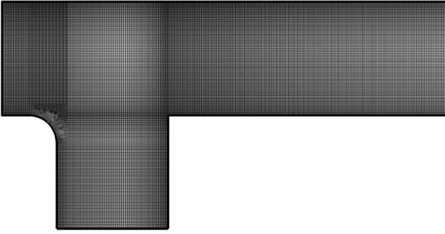
Figure 4: Part of the computational grid close to cavity.
