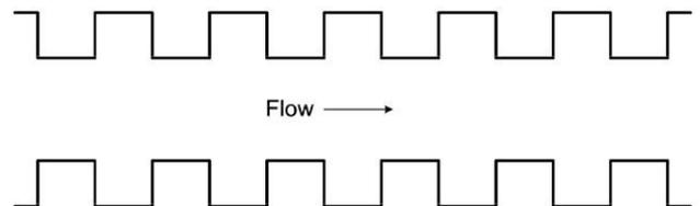
**Figure 1: A typical cross-section of a corrugated pipe with sharp cavity edges.**
