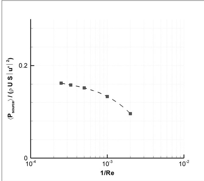
**Figure 6: Reynolds number independency: Reynolds number is plotted against dimensionless average acoustic source power  $\langle P_{\text{source}} \rangle / \rho U S |u'|^2$  at  $St = 0.5$ ,  $|u'_{\text{max}}|/U = 0.2$  and  $r_{\text{up}}/W = 0.25$ .**
