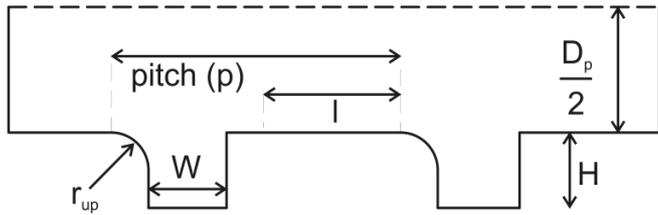
**Figure 2: The geometric parameters of corrugated pipes.**
