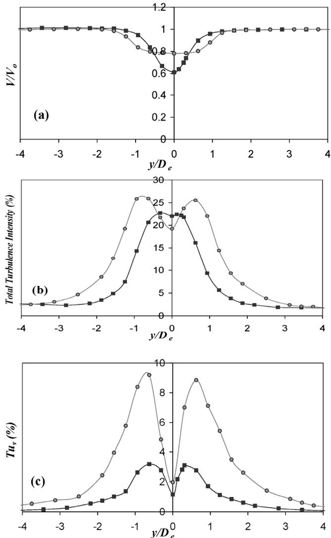
**Figure 9. Wake characteristics for tandem bare cylinders I and finned cylinders II with  $S/D_e = 2$ ; (a) mean velocity profiles; (b) total turbulence intensity profiles; (c) fluctuation velocity at the vortex shedding frequency. Measurements performed at  $x/D_e = 2.5$  and  $V_r = 2.35$  ( $Re = 2.7 \times 10^4$ );  $\blacksquare$ , bare cylinder I;  $\bullet$ , finned cylinder II.**
