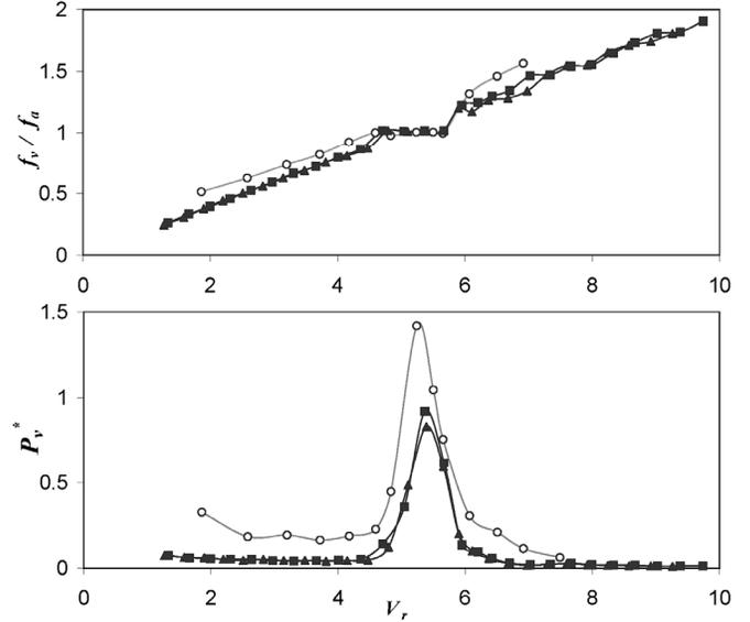
**Figure 3. Frequency ratio ( $f_v/f_a$ ) and the normalized sound pressure ( $P_v^*$ ) as functions of the reduced velocity ( $V_r$ ) for bare single cylinders. ■, bare cylinder I; ▲, bare cylinder II; ○, Blevins and Bressler [16].**
