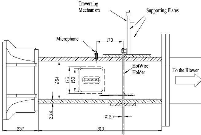
**Figure 1. Details of the test section (All dimensions in mm.)**
