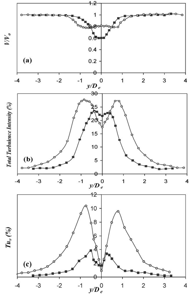
**Figure 7. Wake characteristics for *tandem* bare cylinders I and finned cylinder II with  $S/D_e=1.5$ ; (a) mean velocity profiles; (b) total turbulence intensity profiles; (c) fluctuation velocity at the vortex shedding frequency. Measurements performed at  $x/D_e = 2.5$  and  $V_r = 3.2$  ( $Re = 3.7 \times 10^4$ ); —■—, bare cylinder I; —○—, finned cylinder II.**
