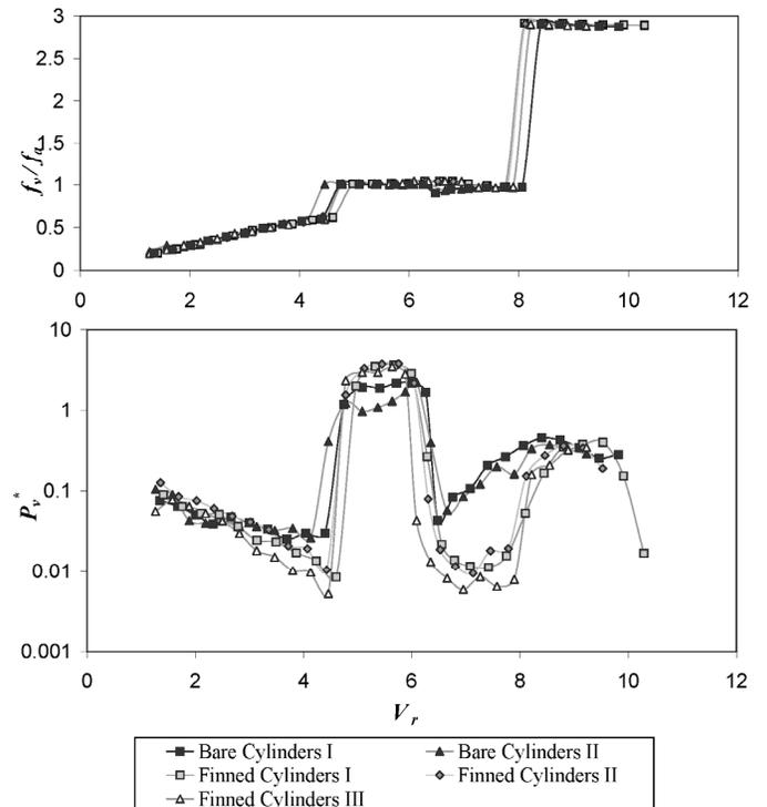
**Figure 10. Frequency ratio ( $f_v/f_a$ ) and the normalized sound pressure ( $P_v^*$ ) as functions of the reduced velocity ( $V_r$ ) for bare and finned tandem cylinders with  $S/D_e = 3$**
