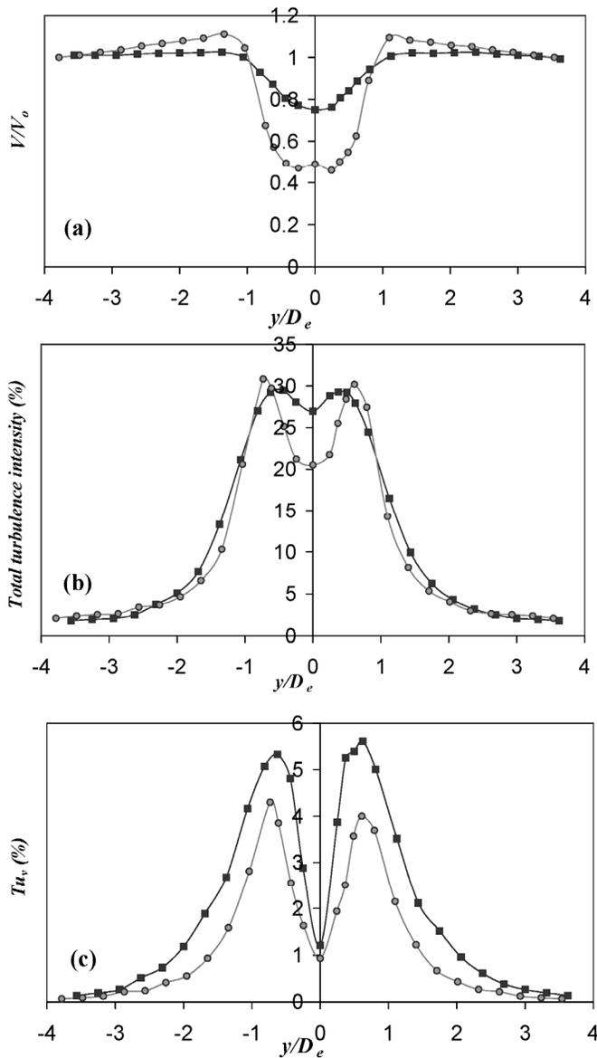
**Figure 5. Wake characteristics for single bare cylinder I and finned cylinder II. (a) mean velocity profiles; (b) total turbulence intensity profiles; (c) fluctuation velocity at the vortex shedding frequency. Measurements performed at  $x/D_e = 2.5$  and  $V_r = 3.2$  ( $Re = 3.7 \times 10^4$ ); —■—, bare cylinder I; —●—, finned cylinder II.**
