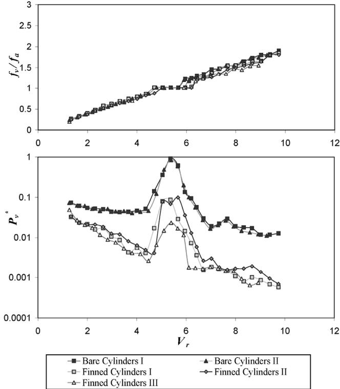
**Figure 4. Acoustic response of the bare and finned single cylinders showing the frequency ratio ( $f_v/f_a$ ) and the normalized sound pressure ( $P_v^*$ ) as functions of the reduced velocity ( $V_r$ )**
