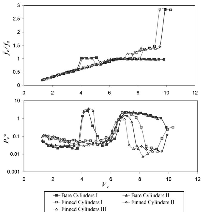
**Figure 8. Frequency ratio ( $f_v/f_a$ ) and the normalized sound pressure ( $P_v$ ) as functions of the reduced velocity ( $V_r$ ) for bare and finned tandem cylinders with  $S/D_e = 2$**
