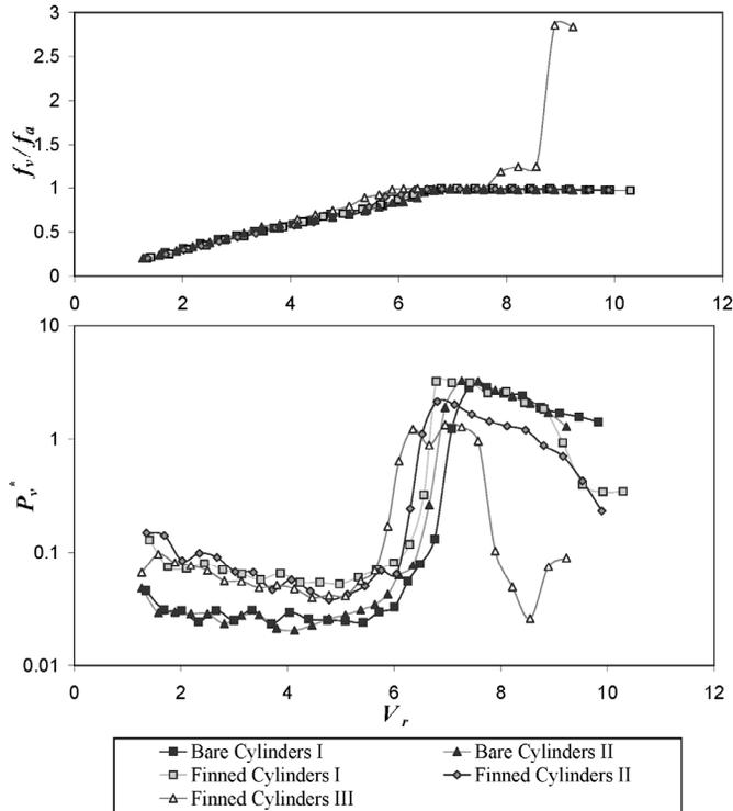
**Figure 6. Frequency ratio ( $f_v/f_a$ ) and the normalized sound pressure ( $P_v$ ) as functions of the reduced velocity ( $V_r$ ) for bare and finned tandem cylinders with  $S/D_e=1.5$**
