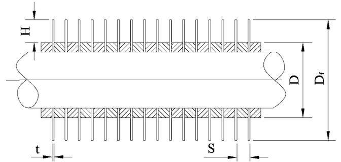
**Figure 2. Details of the finned cylinders**
