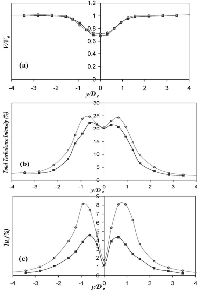
**Figure 11. Wake characteristics for tandem bare cylinders I and finned cylinders II with  $S/D_e=3$ ; (a) mean velocity profiles; (b) total turbulence intensity profiles; (c) fluctuation velocity at the vortex shedding frequency. Measurements performed at  $x/D_e = 2.5$  and  $V_r = 2.35$  ( $Re = 2.7 \times 10^4$ ); —■—, bare cylinder I; —●—, finned cylinder II.**
