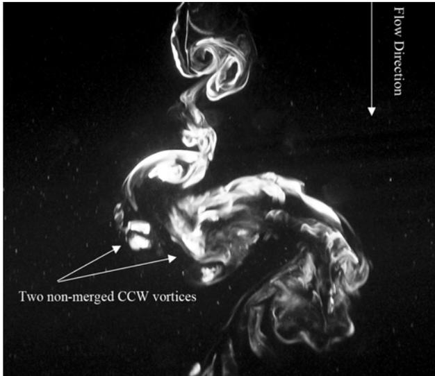
FIG. 14 2P-LIKE SHEDDING PATTERN FOR CASE A1, ( $U^*=6.6$ ,  $Z/L=-0.65$ , AND  $\zeta_Y=0.45\%$ ).
