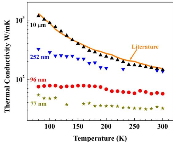
**Fig. 1** Temperature dependent effective thermal conductivity of silicon substrates as measured by heater wires of widths 10 μm, 252 nm, 96 nm and 77 nm in the temperature range 300 - 80 K [1]. The reported literature value of the thermal conductivity of silicon is plotted for comparison. Up to two orders of magnitude reduction in the effective substrate thermal conductivity occurs due to the size-effect of nanoscale heat source.
