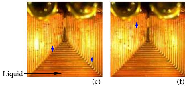
**Figure 8.** Consecutive pictures of flow boiling in straight passages heat exchanger with 10 ms interval from (a) to (f)
