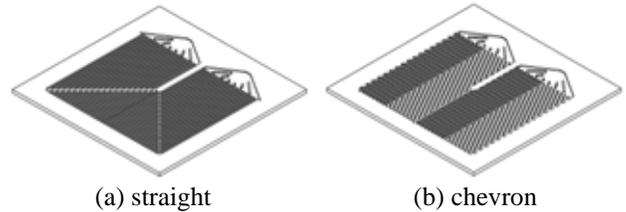
**Figure 2.** Flow passage patterns of heat exchangers in the present study.
