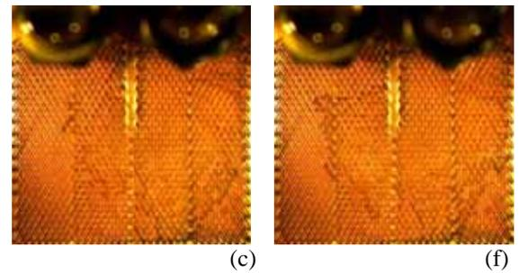
**Figure 9.** Consecutive pictures of flow boiling in chevron passages heat exchanger with 30 ms interval from (a) to (f)
