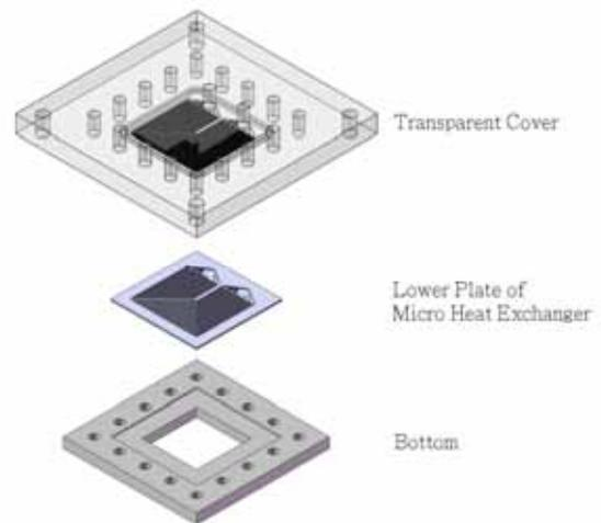
**Figure 3.** Test section assembly for flow visualization
