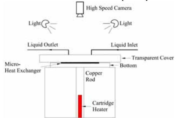
**Figure 5.** Schematic diagram of the visualization experimental apparatus
