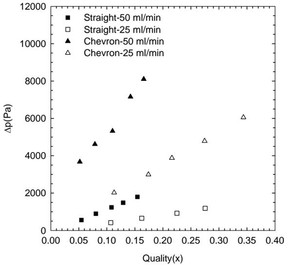
**Figure 6.** Pressure drop at various flow rate and exit vapor quality in heat exchangers
