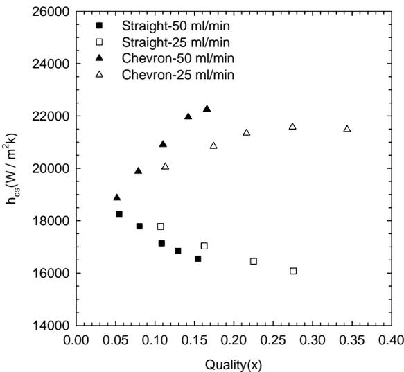
**Figure 7.** Heat transfer coefficient and vapor quality relation for different micro heat exchangers
