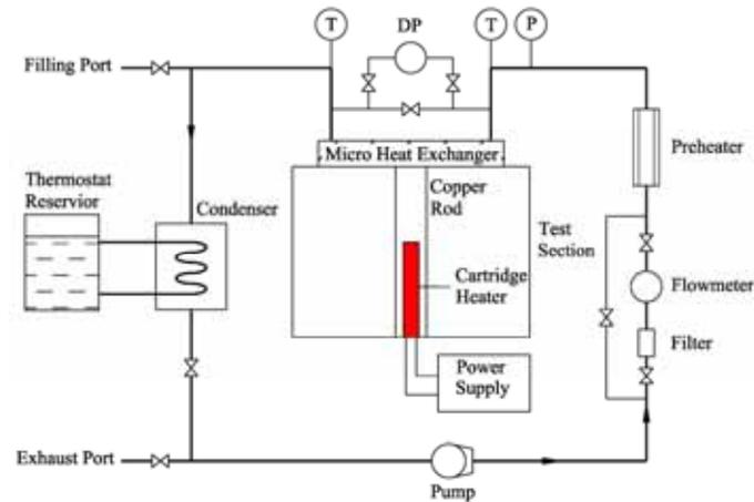
**Figure 4.** Schematic diagram of the heat transfer performance test apparatus
