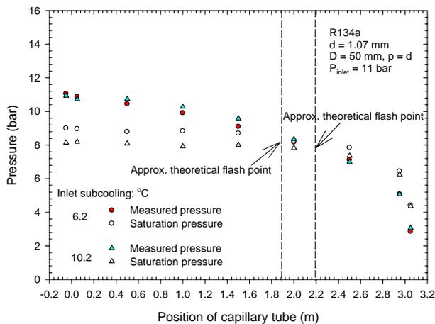
**Fig. 6:** Pressure distribution at various degrees of subcooling
