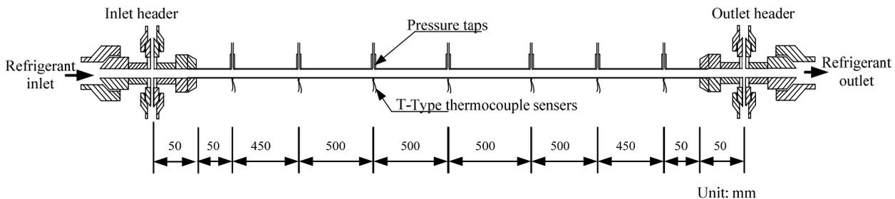
**Fig. 2: Schematic diagram of the test section**
