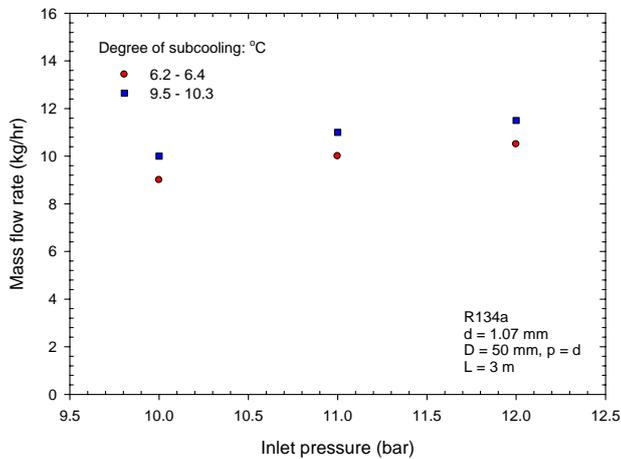
**Fig. 7:** Effect of inlet pressure on the mass flow rate
