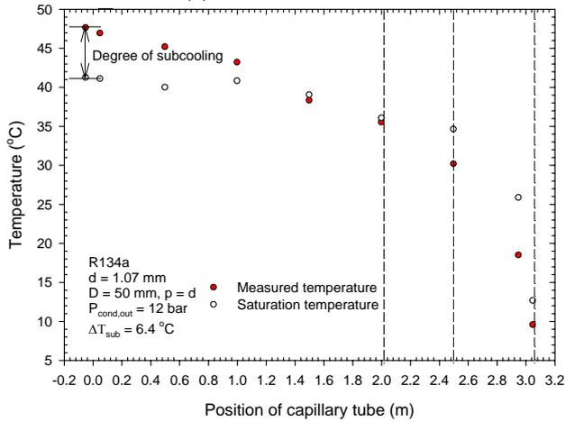
**Fig. 3** Flow phenomena inside the capillary tube (a) pressure distribution, (b) temperature distribution
