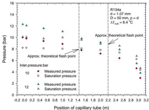
**Fig. 4:** Pressure distribution at various inlet pressures
