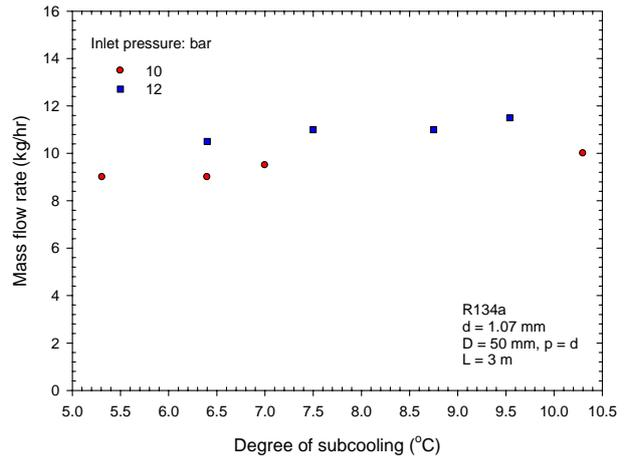
**Fig. 5:** Effect of inlet pressure on the mass flow rate
