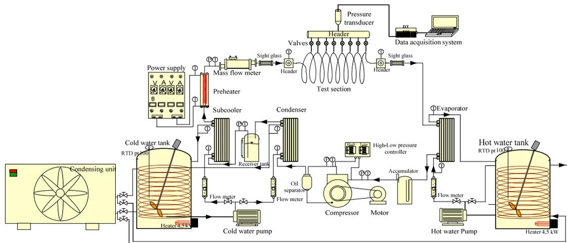
**Fig. 1: Schematic diagrams of the experimental apparatus**
