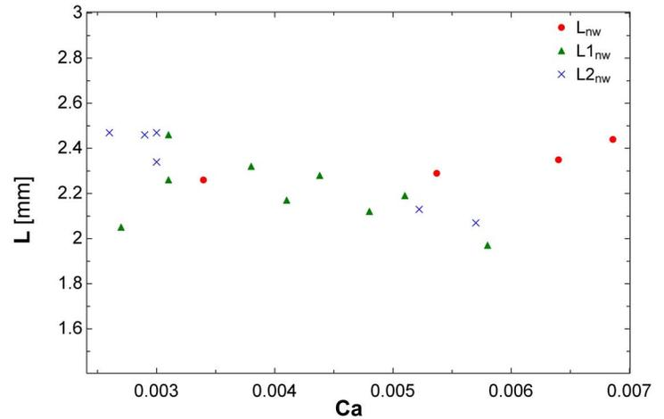
Figure 11: Transition Length vs.  $Ca$ .  $L_{nw}$ ,  $L_{1nw}$  and  $L_{2nw}$  represent the distance between the contact line and the hydraulic jump when first observed (measured in three test runs).
