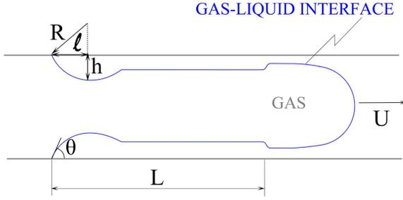
Figure 7: Non-Wetting Film Deposition with Hydraulic Jump
