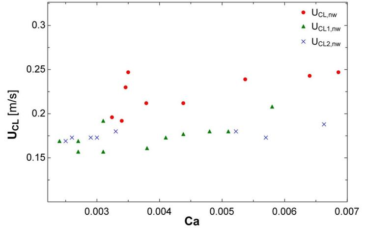
Figure 10: Contact Line Velocity vs.  $Ca$ .  $U_{CL,nw}$ ,  $U_{CL1,nw}$  and  $U_{CL2,nw}$  are contact line velocities measured in the non-wetting tube in three test runs.
