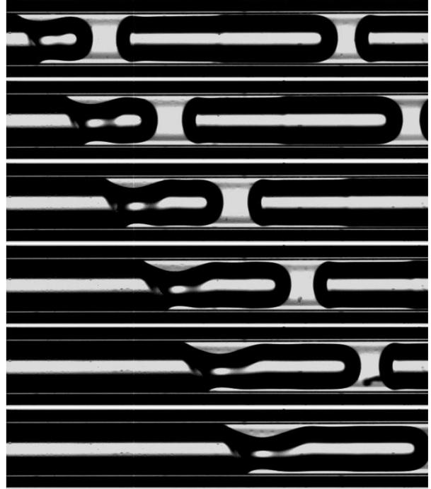
Figure 6: Non-wetting Supercritical Taylor bubble (with shock),  $Ca = 0.0035$ . Images 2 ms apart. The width of the images is 5.735 mm.
