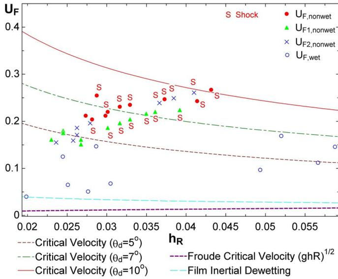
Figure 9: Front Velocity vs. Nondimensional Film Thickness.  $U_{F,nonwet}$ ,  $U_{F1,nonwet}$  and  $U_{F2,nonwet}$  are wave front velocities measured in three separate runs with the non-wetting test section.  $U_{F,wet}$  is taken in the wetting tube.
