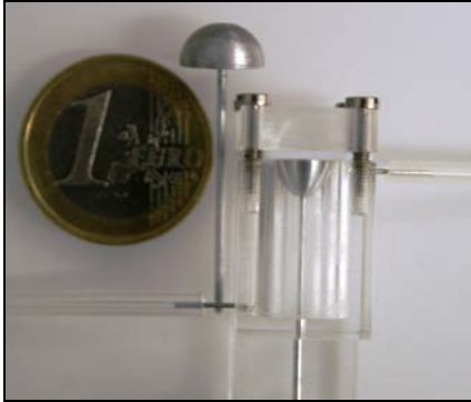
Figure 2: The fabricated minipump based on the dynamic rectifying geometries; please see the two plungers that are used to realize the bidirectional pumping
