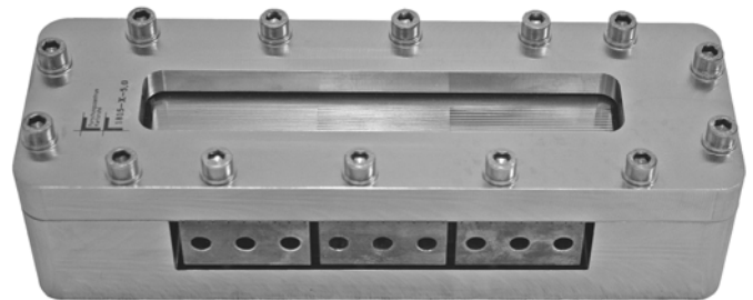
Figure 1: Test device; electrically powered evaporator with a glass window for optical investigation and exchangeable microstructured metal foils.
