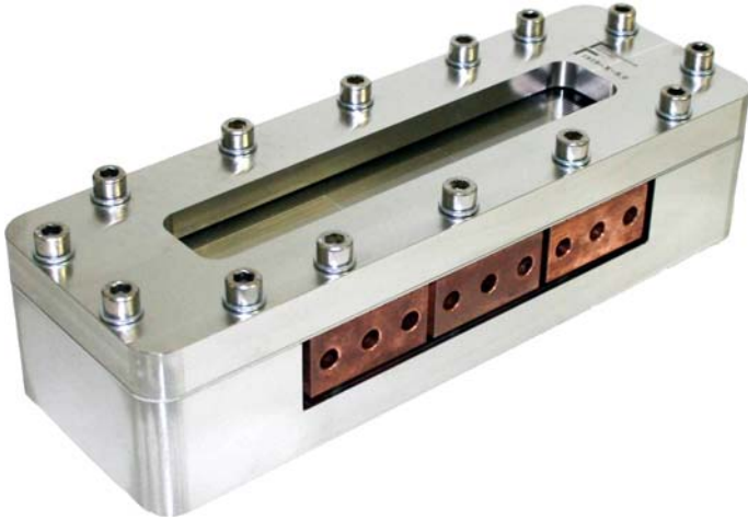
Figure 4: Electrically powered microstructure device, providing exchangeable micro channel foils and a glass lid for high speed videography.
