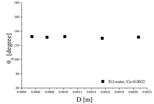
Figure.8  $\theta_A$  of various channel diameters
