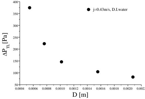
Figure.4  $\Delta P_{TL}$  of various channel diameters
