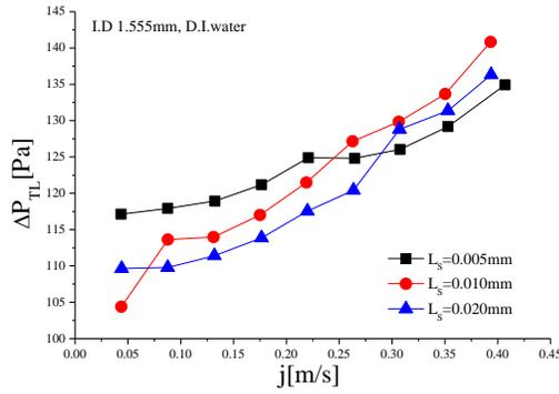
Figure.3  $\Delta P_{TL}$  of various lengths of liquid slug
