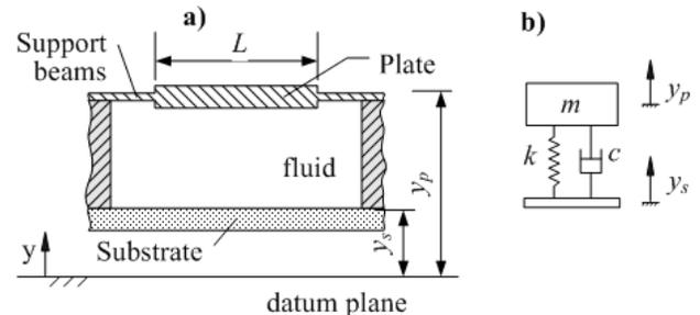
**Fig. 1. a) Elastically supported, free-standing plate. Sinusoidal displacement is imposed on substrate. b) Schematic of system idealized as single degree-of-freedom.**
