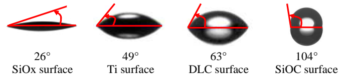
Figure 8. Static contact angles of a water-droplet on the sample surfaces at room temperature.
