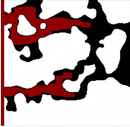
FIGURE 6. Displacement of resident oil (black) by injected water (red) after 112500 time steps.
