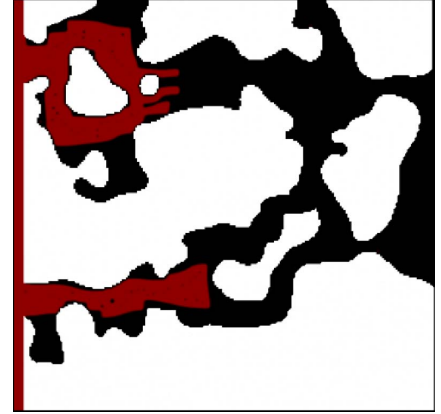
FIGURE 5. Displacement of resident oil (black) by injected water (red) after 75000 time steps.
