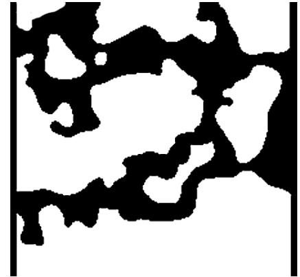
FIGURE 2. Final image of a section of the original image obtained after processing. Black region depicts pore space and white region depicts solid grains.
