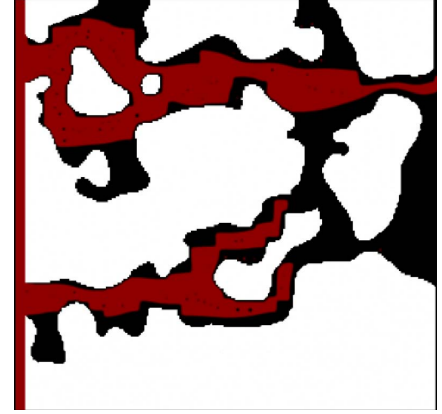
FIGURE 7. Displacement of resident oil (black) by injected water (red) after 150000 time steps.
