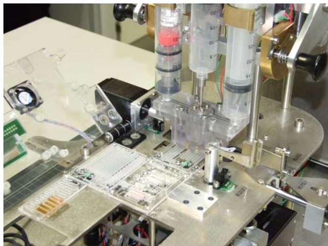
Fig. 4 Microsystem for automated isolation of circulating tumor cells from whole blood samples based on disposable polymer chips. The chip system comprises an incubation module, an amplification module, a buffer storage module and a detection module. The operating device shows all mechanical and electronic components needed for process control.
