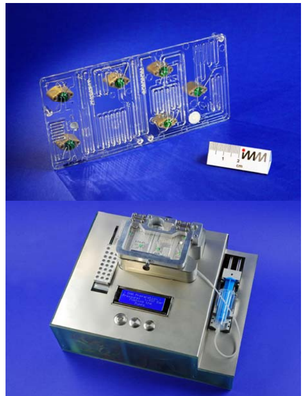
Fig. 1 Microfluidic chip-based system for isolation and lysis of bacteria followed by nucleic acid purification. The disposable chip (top) shows filters for cell accumulation and DNA binding, Kenics mixers, buffer reservoir channels and turning valves for connecting channels. The operational device (bottom) contains electronics for process control on chip including heaters. Fluid transport is realized by a syringe pump.
