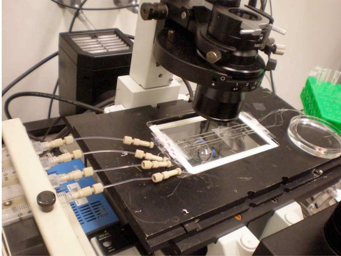
**Figure 1.** Experimental setup on IX81 microscope stage. Syringe pump on left controls flow rate, and connectors and larger tubing connect syringes to microtubes on microscope stage. The right-hand ends of the microtubes are placed in samples, to be withdrawn through the tube.
