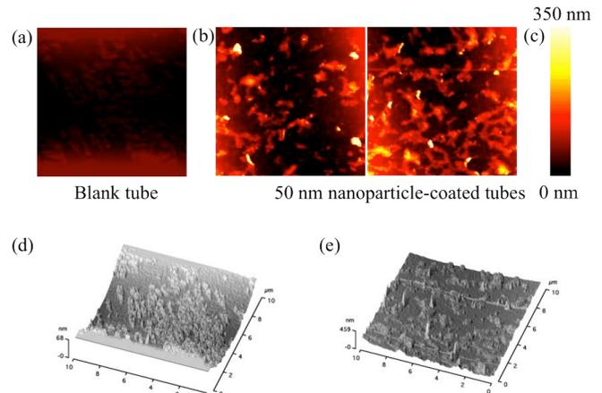
**Figure 2.** Atomic Force Microscopy Images of Tube Surface. (a) Blank tube, with no nanoparticles. (b) Two locations of a tube coated with nanoparticles. (c) Thermal scale for images in (a) and (b). Three-dimensional representations of (a) and (b) are shown in (d) and (e).
