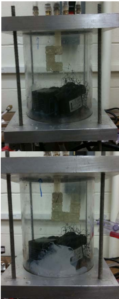
Figure 6: Docking and proper alignment of cube using suction enhancement and solenoid based sink-cycling. Cube shown in image is the one from the upper right corner of Figure 1.
