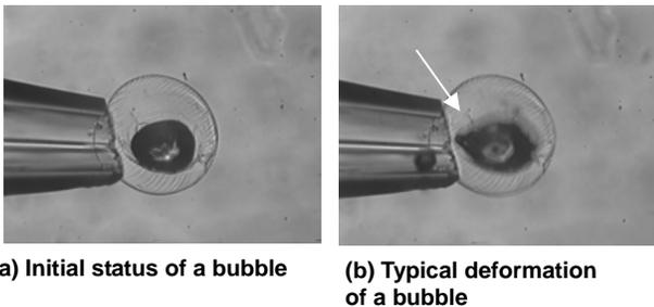
Fig. 5 Bubble deformation inside a capsule (43kHz)
