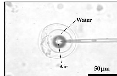
Fig.1 Prototype of microcapsule including gas and liquid
