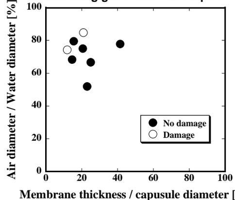
Fig.3 Geometrical mapping between membrane thickness and air diameter of microcapsule
