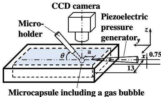
Fig. 4 Experimental apparatus for observation of deformation process of a bubble inside a capsule
