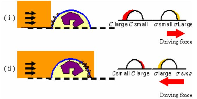
**Fig.12** Concept of driving force by alternative change of concentration gradient on the membrane; (i) first stage, the concentration is high at front (ii) second stage, the concentration is high at the end
