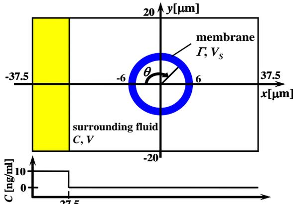
**Fig.10** Computational model for analyzing the transport process of concentration around the neutrophile with membrane and initial concentration profile along x axis
