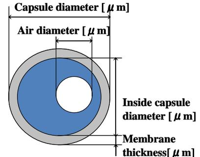
Fig.2 Parameter of geometry for the microcapsule including gas bubble and liquid
