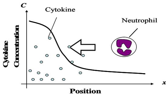
**Fig. 7 Concept of chemotaxis using concentration Marangoni effect**
