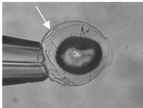
Fig. 6 Bubble deformation inside a capsule (77kHz) when the gas diameter ratio to diameter of capsule is almost 1.0
