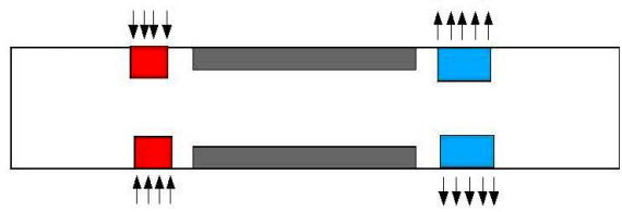
FIGURE 3. Heat exchangers - constant prescribed heat
