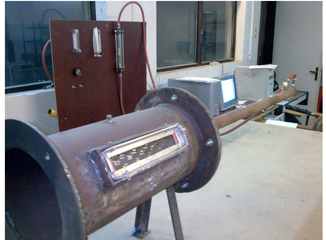
Figure 3. EXPERIMENTAL COMBUSTION CHAMBER SETUP
