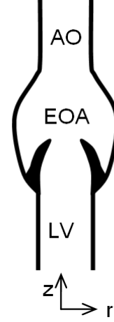
Figure 1. Schematic of the flow across an aortic valve. LV: Left Ventricle, AO: Aorta, EOA: Effective Orifice Area
