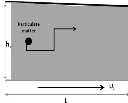
**FIGURE 2.** A SCHEMATIC OF THE MODEL GEOMETRY THAT WE USE IN OUR STUDY. IN THIS PAPER, THE UPPER PLATE IS HELD FIXED WHILE THE BOTTOM IS TAKEN TO BE MOVING IN KEEPING WITH THE CONVENTION IN PREVIOUS PAPERS.
