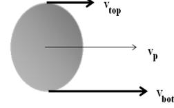
**FIGURE 5.** A SCHEMATIC OF THE LOCAL SHEAR LAYER IN THE NEIGHBORHOOD OF THE PARTICLE. THE RESULTING SHEARING FORCE INDUCES A COUNTERCLOCKWISE ROTATION THUS GIVING THE PARTICLE A LIFT FORCE.
