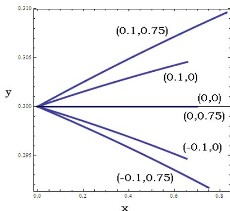
**FIGURE 6.** THE PLOT SHOWS PARTICLE TRAJECTORIES OVER TIME FOR DIFFERENT  $M$  AND  $De$ . THE INITIAL VELOCITY OF THE PARTICLE IS TAKEN TO BE HALF THE VELOCITY OF THE FLUID AT THE INITIAL POSITION, DIAMETER,  $D = 0.1$ ,  $S = 1.1$ . THE LABELS MENTIONED ALONGSIDE THE TRAJECTORIES INDICATE  $(M, De)$ .
