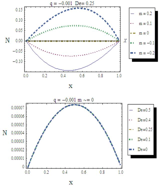
**FIGURE 4.** THE PLOT SHOWS THE VARIATION IN THE NORMAL STRESS,  $N = T_{YY}$ , UPON THE BOTTOM PLATE AS A FUNCTION OF  $X$ , SLOPE  $M$  AND  $De$ . IN THE UPPER FRAME WE FIX  $De = 0.25$  AND  $Q = -0.001$  AND WE SEE THE STRESS VARIATION IN  $X$  WITH THE RESPECT TO THE SLOPE OF THE PLATES. IN THE LOWER FRAME WE SHOW THE VARIATION IN NORMAL STRESS WITH  $De$ .
