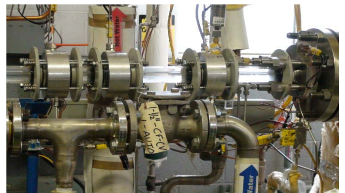
Figure 7. Portion of glass test section; glass sections are separated by instrumentation rings that house thermocouples; the flange on far right is inlet flange to reservoir—see Figure 6.
