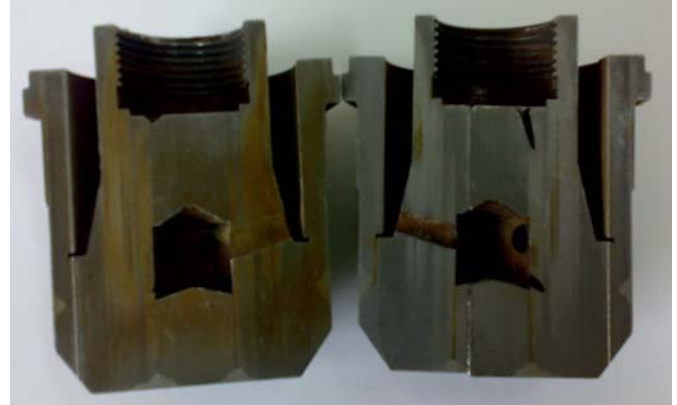
Figure 1. Longitudinal cross section of the sample nozzle
