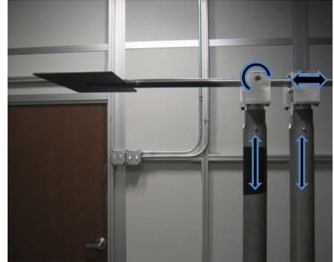
**Figure 1.** Dynamic Pitch-Plunge Rig
