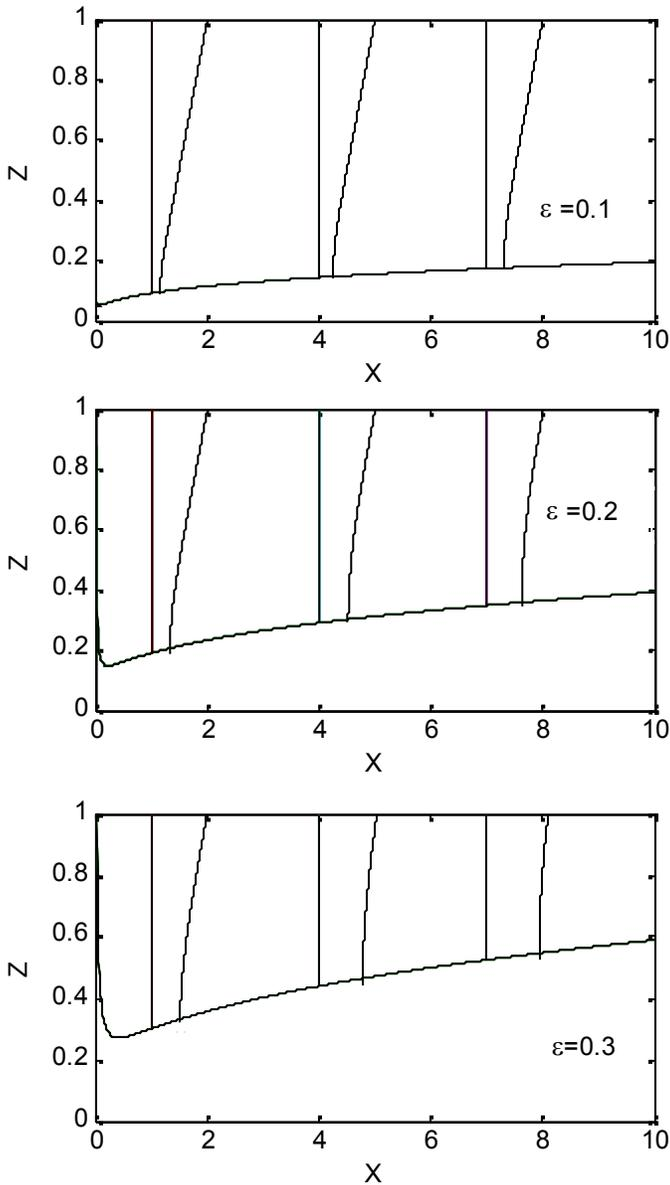
**FIGURE 6: STREAM WISE VELOCITY VERSUS POSITION X FOR  $\epsilon = 0.1, 0.2,$  and  $0.3$**
