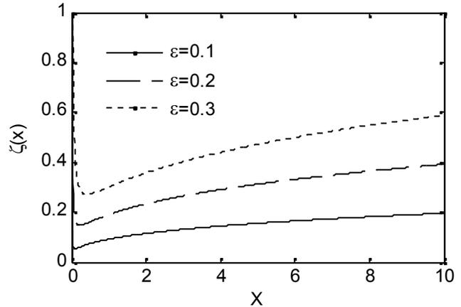
**FIGURE 4: FREE SURFACE HEIGHT  $\zeta(x)$  VERSUS POSITION  $x$  AT DIFFERENT  $\varepsilon$**
