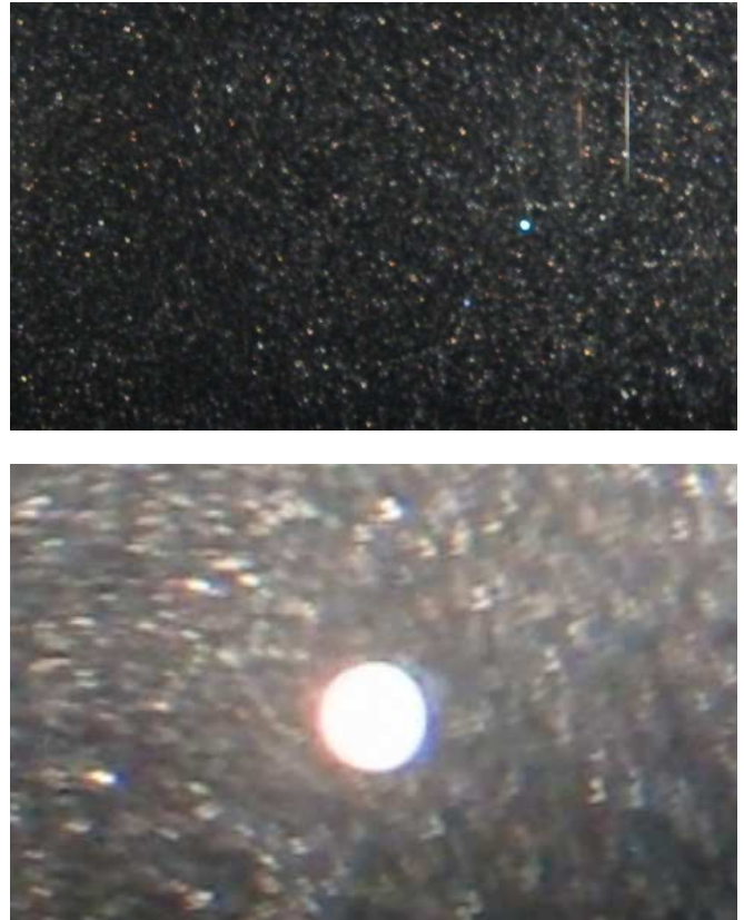
Figure 6. a) Colored scattered light from particles of around 25 \mu\text{m} diameter. b) Colored scattered light from a sphere of 5 mm diameter.
