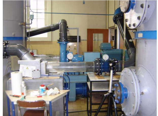
Figure 4. Scheme of the DynFluid axial pump test-ring.
