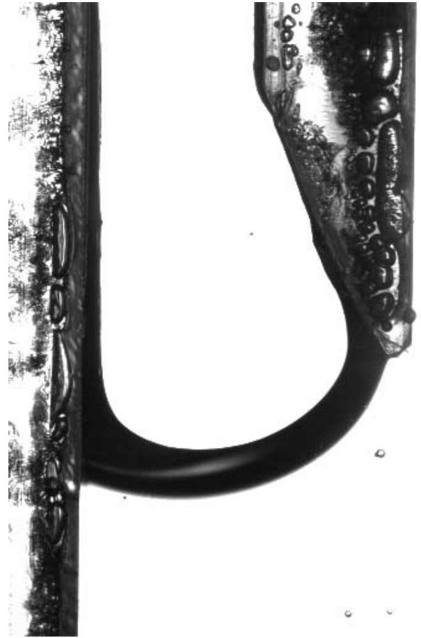
FIGURE 11. WATER-AIR MENISCUS UNDERNEATH THE STEP DURING A NATURAL FREQUENCY TEST. THE STEP HEIGHT IS 3.5 mm FOR COMPARISON.
