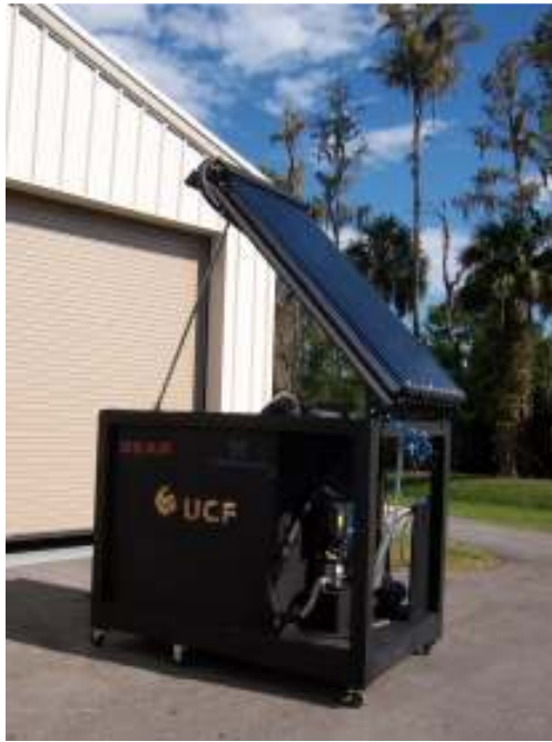
Figure 4: Solar Collector and Storage
