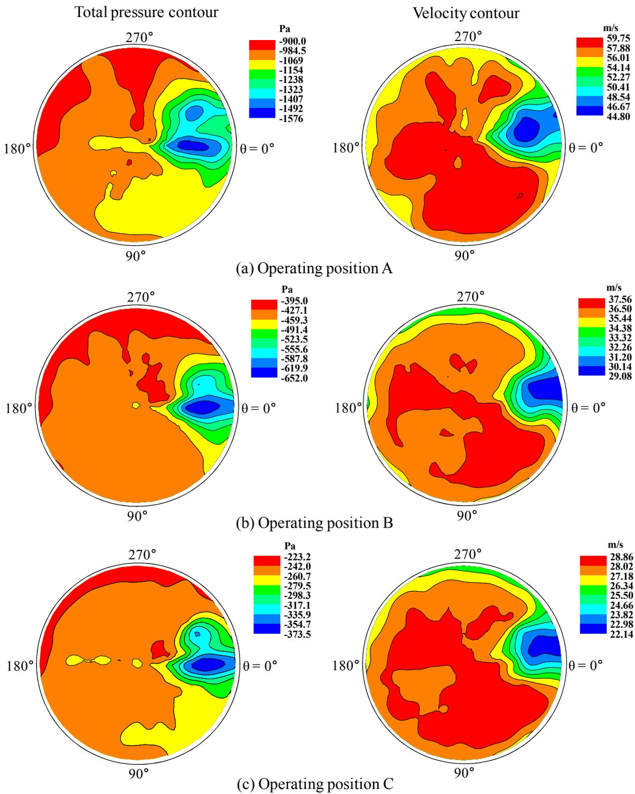
**Figure. 7** Total pressure and velocity contour at different flow rate
