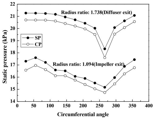
Figure. 3 Static pressure distribution in vaneless diffuser
