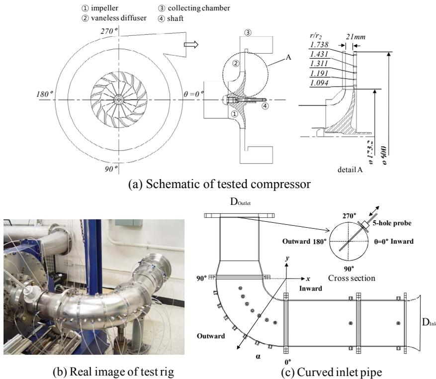
**Figure. 1** Test rig with curved inlet pipe (a) Schematic of tested compressor (b) real image of test rig (c) curved inlet pipe
