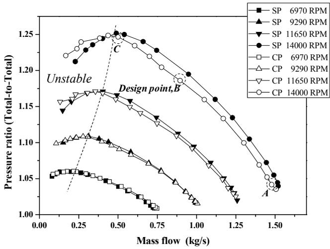
Figure. 2 Performance of a tested centrifugal compressor
