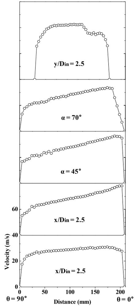
Figure. 4 Streamwise velocity profile at design point B
