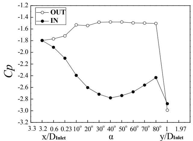
Figure. 5 Distribution of wall static pressure at operating point B
