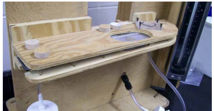
Figure 2. Schematic of the laminar flow wind tunnel.
