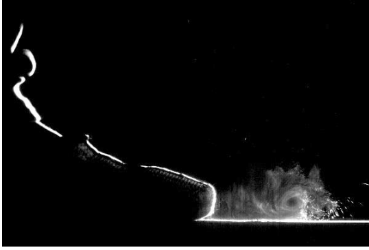
FIGURE 5: PARTICLES FLOW VISUALIZATION WITH AN ACTUAL FOOT STOMPING OF TOE.
