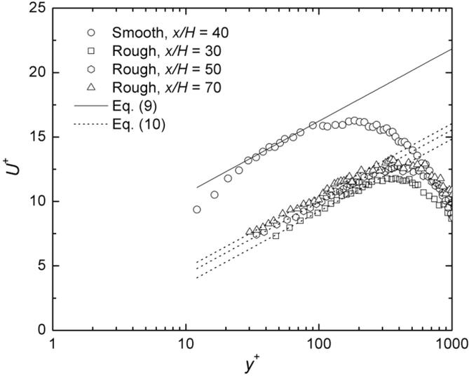
**FIGURE 4.** MEAN VELOCITY PROFILES OF A ROUGH TURBULENT WALL JET IN INNER COORDINATES.
