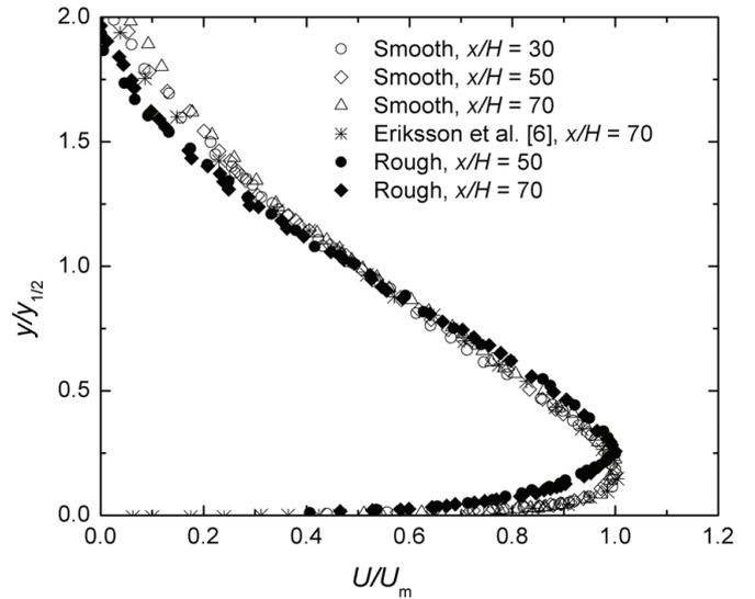
FIGURE 3. MEAN VELOCITY PROFILES OF SMOOTH AND ROUGH WALL JETS IN OUTER COORDINATES.
