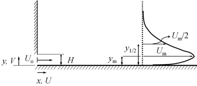
**FIGURE 1.** SCHEMATIC OF A TURBULENT WALL JET.
