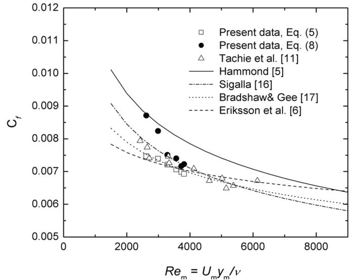
FIGURE 2. SKIN FRICTION COEFFICIENT AS A FUNCTION OF REYNOLDS NUMBER FOR A SMOOTH TURBULENT WALL JET.
