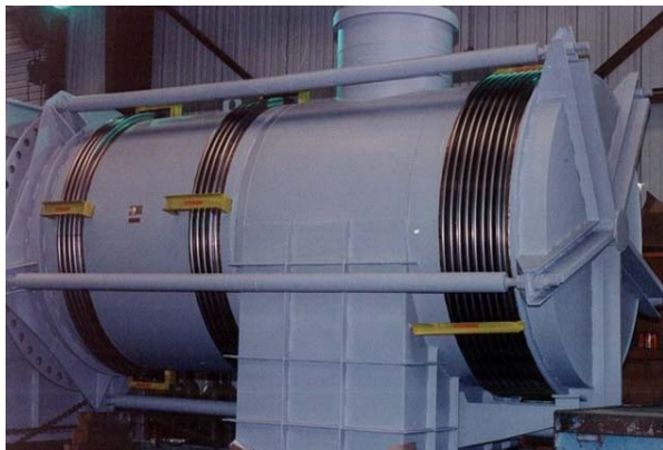
Figure 2: Part of the Studied System – Hood-Bellows
