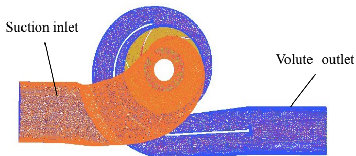
Fig.2 Grid of vacuum tower bottom pump model
